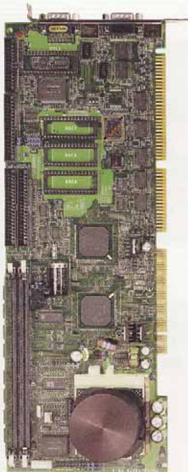
Pentium ISA/PCI single-board computer with watchdog timer for supervising program execution.
